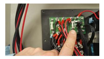
This is the location of the Charger Fuse. Gently lift the fuse using a non-scratching tool, e.g. a wooden pencil. Do not use metal tools! You could harm the Printed Circuit Board (PCB) underneath the fuse. If the fuse is gone, replace it (G 1.6A 250V 5x20mm slow type). If you are not sure whether the Charger Fuse is gone or not, use a common multimeter to test the fuse for continuity. If you cannot find continuity, the fuse is gone and needs to be replaced.
