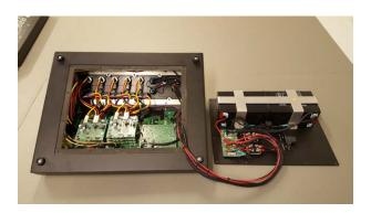
Lay down the housing next to the bottom plate as shown in the image above.
