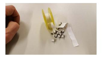
Now pick up the prepared screws with the <u>fresh</u> PTFE tape.
