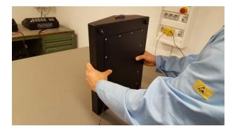
Put the device horizontal like shown in the image above. Ensure you strongly press the bottom plat with the thumbs.
