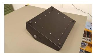
Use the prepared screws wrapped with PTFE Thread Seal Tape to close the Field Controller. ATTENTION: Not using the PTFE Seal Tape will render the warranty void and the liability will be exclude
