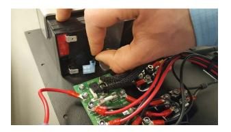
Unplug the fused Battery Interconnection Cable from the negative pole of the left hand side battery. Be careful to not harm the PCB board next to it and the cables connected to it.
