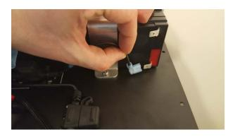
Unplug the fused Battery Interconnection Cable from the positive pole of the right hand side battery.
