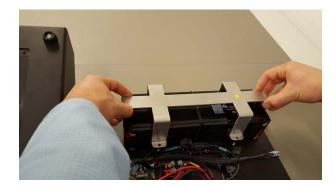
Lift off the holder. The batteries are free now.
