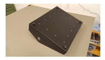
Place the Field Controller bottom up on an ESD safe underground, e.g. an ESD mat. Ensure the ESD mat has a proper 1 MOhm connection to earth ground. Now, unscrew all 14 bottom screws.
