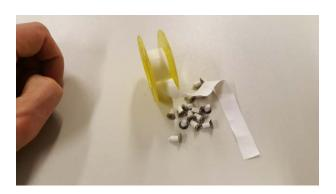
In order to seal the threads of the screws, you need to refresh the PTFE Thread Seal Tape on the screws. The PFTE Thread Seal Tape (also know as Teflon Seal Tape) can be purchased in every usual hardware store. Prepare the screws as you will need them in the following steps.
