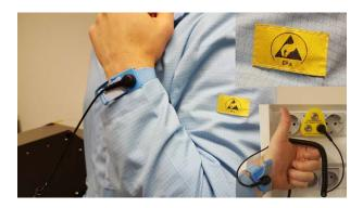
Always ensure to work in an ESD safe environment whenever the Pyrodigital<sup>®</sup> Field Controller Model A needs to be opened or is open! Properly ground yourself and the ESD mat underneath the device. Never open the Pyrodigital<sup>®</sup> Field Controller Model A outside of an EDS safe environment. Please ask Innovative Pyrotechnik GmbH or your local vendor for advice, if you are unsure about EDS safe environments.
