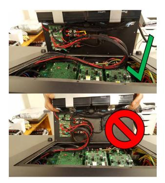
Ensure the cable harness is not twisted! The cable harness must lay like in the upper part of this figure and must not be curled up like in the lower part of this figure.
