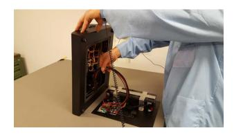
Make sure the cabling is loose enough so you can proceed to lay down also the housing itself. The cables might be hidden in the compartment in front of the main board.
