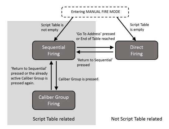
After entering the MANUAL FIRE MODE the Field Controller checks if the selected Script Table is empty. If so, the Field Controller enters Direct Firing. In case the Script Table is not empty, the Field Controller enters Sequential Firing.
