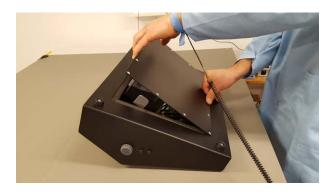
Now slowly lower the bottom plate towards the main housing. Use one hand to support the bottom plate on its edge. This prevents that the bottom plate slips off. Ensure you do not jam any cables during closing.
