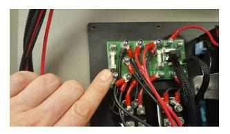
In case you need a fuse to replace the Charger fuse, you can find a SPARE FUSE at this position on the PCB. Take this fuse and put it into the holder of the Charger Fuse. Do not forget to refill the SPARE FUSE holder, so you always have a spare with you. Note: The fuse in the spare holder is only a spare part. It is not connected to any circuitry. It is only purpose is to provide a spare fuse when needed urgently.
