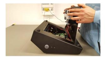
Place the bottom part with its edge horizontally on the lower edge of the frame of the bottom opening of the device, like shown in this image.
