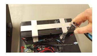
Unscrew the battery holder. Use a socket SW 7mm to open the M4 nuts.
