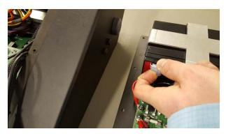
Unplug the Battery Plus Cable from the positive pole of the left hand side battery.
