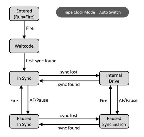
First the Operator has to depress FIRE to proceed to the 'Waitcode' state. Then, after the first valid timecode frame is received, the clock is 'In Sync' to the timecode. If the timecode gets lost or invalid ('sync lost'), the clock switches over to the internal clock source 'Internal Drive'. When the timecode resumes (and is valid), the clock is resynchronized and again 'In Sync'.
