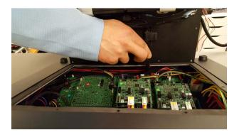
Ensure that the cables connecting the bottom plate and the main housing are safely stored in the compartment in front of the mainboard. Ensure the cabling does not press on the circuit boards when closing and that no cables are jammed between bottom plate and main housing when closing the Field Controller.
